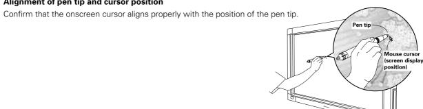
If the cursor position differs from that of the physical pen tip, adjust as follows:
